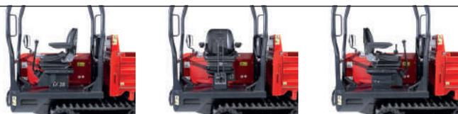
▶ The comfortable seat can rotate 180 degrees to allow to steer the machine with maximum visibility in both directions.
