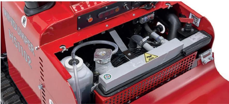
◀ The new housing is designed to allow a simple inspection/routine maintenance thanks to the improved engine access.
