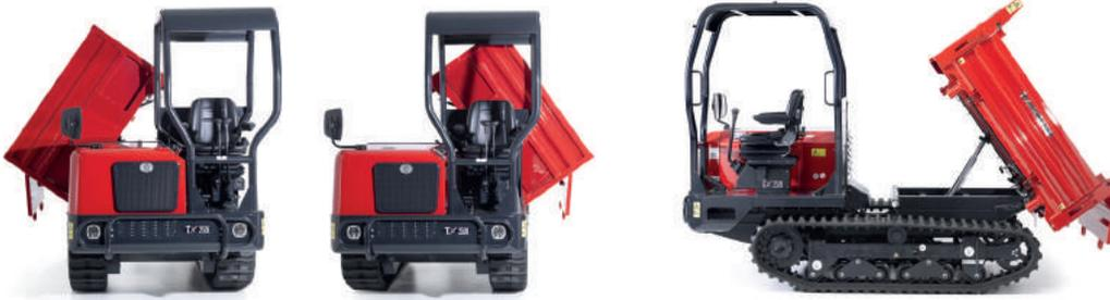
Triple flange rollers are designed to make TX2500 drive safe on slopes and rough terrain, as they ensure stability and reduce the risk of untracking. The short pitch offers smooth drive for optimal comfort at high speed.
